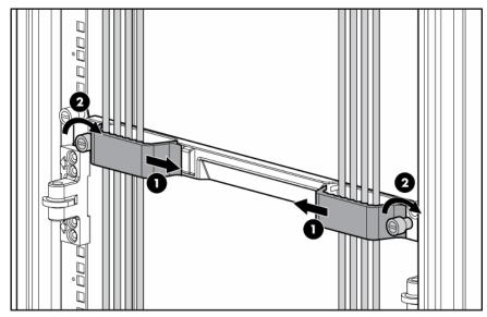
Tighten the thumbscrew to secure the cable retaining bracket over the cables (2).
